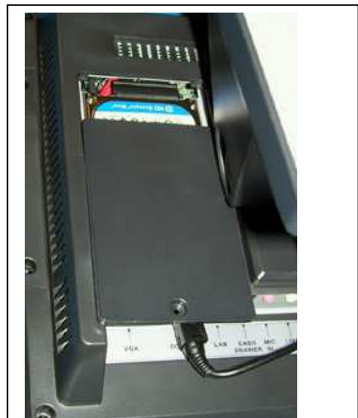
Figure 4, HDD seen under the opened door
