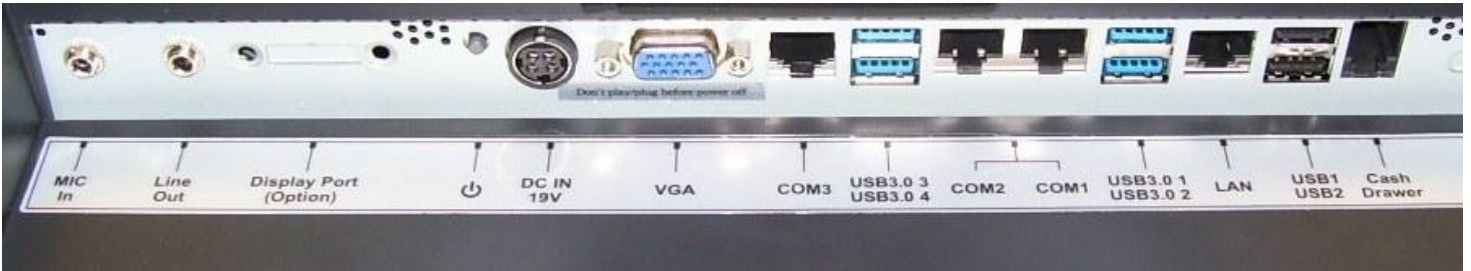
Figure 2, 2190 POS I/O Panel
