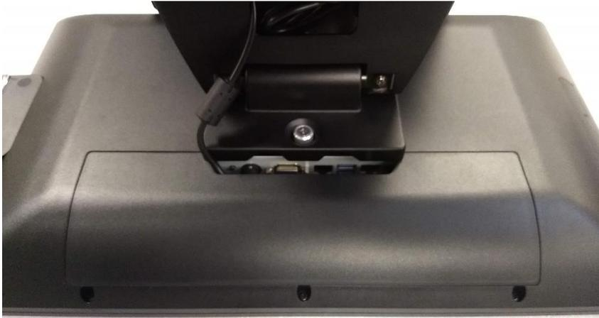
Next remove the four base adapters using a flat-bladed screwdriver. The photo below shows two of the adapters removed. A VESA bracket can now be mounted to the 2600 using appropriate length metric M4-0.7 screws.
