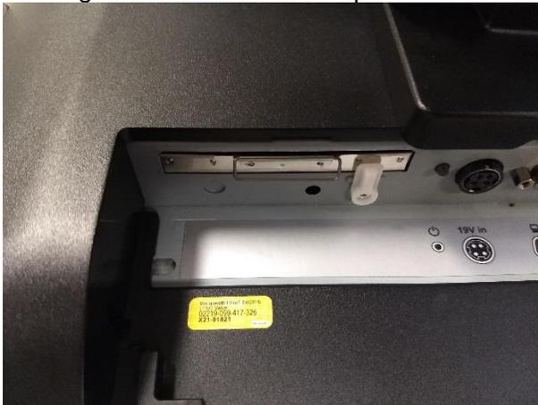
Locking tab – rotated for drive removal
