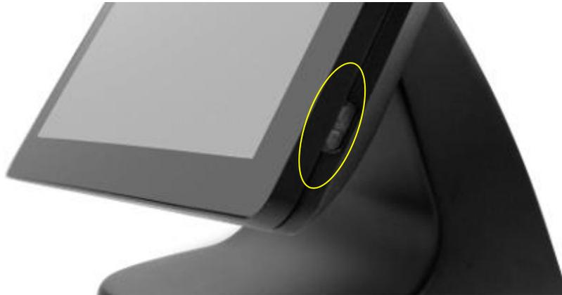
The 2600 has a projected capacitive multi-touch screen that has been factory calibrated and will not require any additional driver installation when used with most current operating systems, such as Windows 10.
