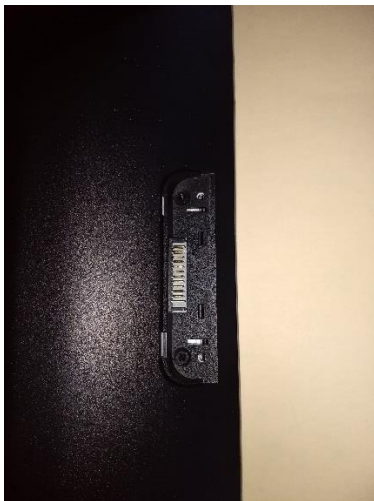
MSR connector cover removed
