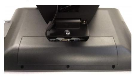
Next remove the four base adapters using a flat-bladed screwdriver. The photo below shows two of the adapters removed. A VESA bracket can now be mounted to the 2670 using appropriate length metric M4-0.7 screws.
