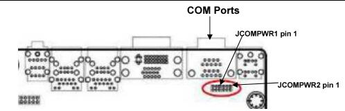
JCOMPWR1: Selects RI or voltage output for COM1 DB9 pin 9 JCOMPWR2: Selects RI or voltage output for COM2 DB9 pin 9
