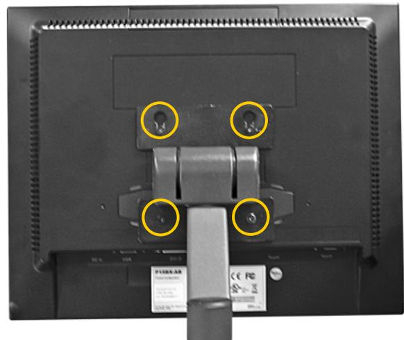
**WARNING! Make sure that the four mounting screws for the LCD monitor are SECURELY fastened! Failure to do so will cause mechanical damage to the monitor!**
