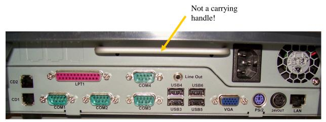
WARNING: To avoid accidental power-up during installation, connect the AC Power Cable last.
