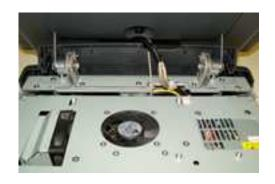
Pivot the cover up; unplug the power connector by pressing its tab and pulling it out of the motherboard jack. Raise the cover fully; aligning the pivot screws in the chassis slots and locking the rear cover up at a 45° angle.
