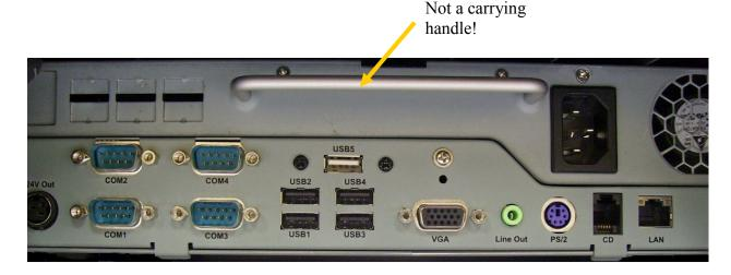
Note: If you find that the supplied AC power cable interferes with your ability to connect a 15-pin VGA plug to the I/O Panel's Video jack, substitute a standard straight PC power cord for the supplied 90° cord.
